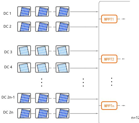
Prior to connecting the inverter to PV inputs, the specifications in the following table should be met:
