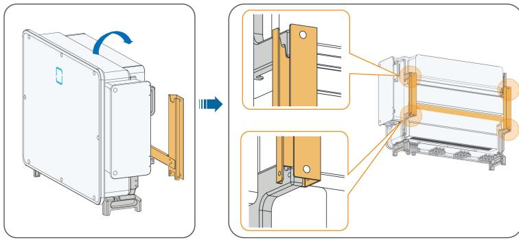
step 3 Fix the inverter with screws.
