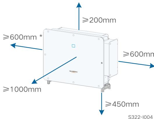
\* In case this distance is less than the distance in the diagram, move the inverter from the mounting-bracket or wall before maintaining fans.
