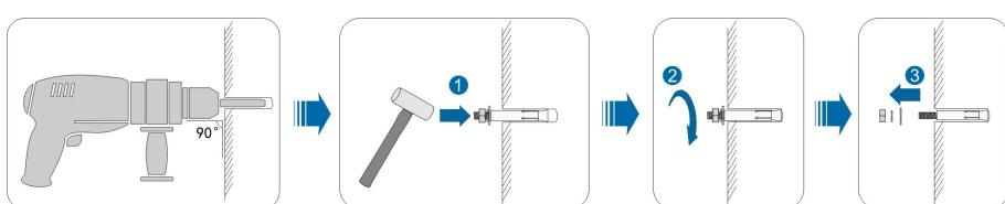
step 4 Fix the mounting-bracket with the expansion bolts.
