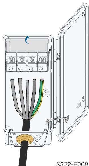
step 7 Connect cables with crimped OT/DT terminals to corresponding terminals and secure them.
