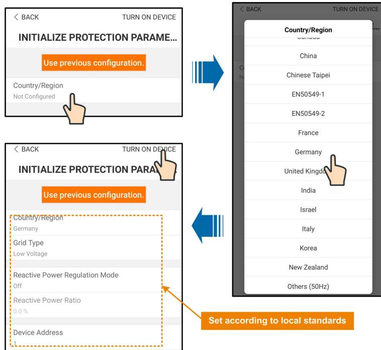
figure 7-3 Initialization Protection Parameter
