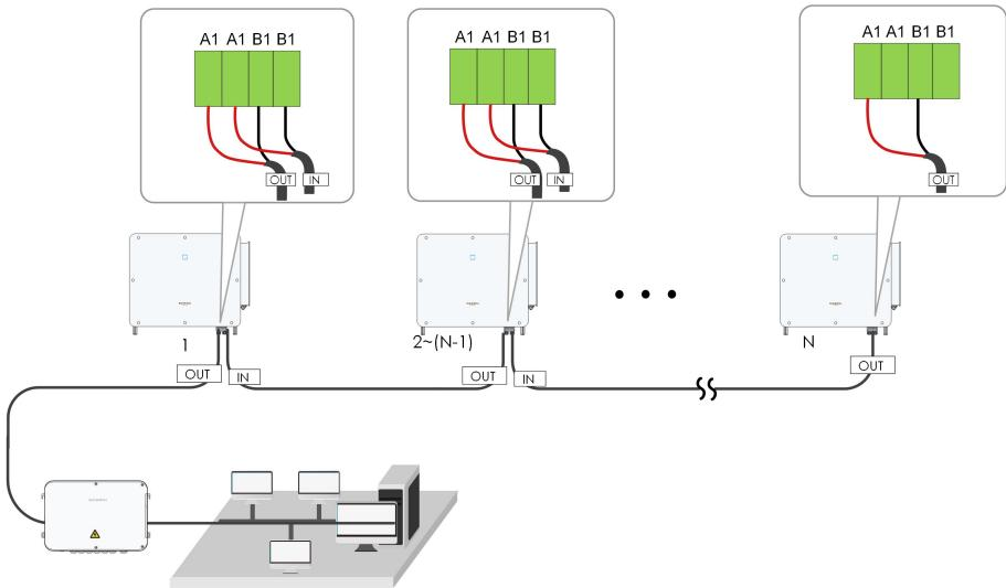
figure 5-5 Multi-inverter Communication System 【RS485\_1 interface (terminal block)】
