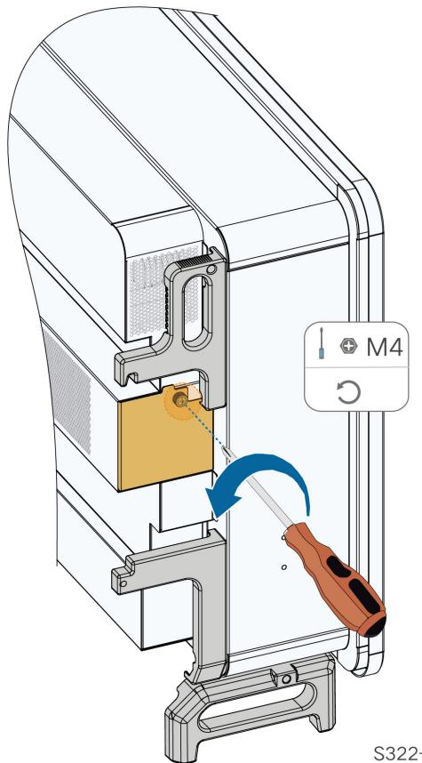
step 3 Press the tab of the latch hook, unplug the cable connection joint outwards, and loosen the screw on the fan holder.
