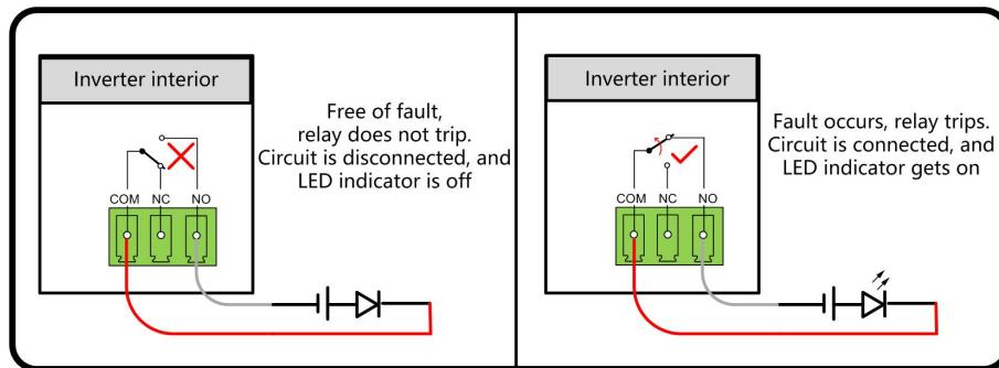
figure 5-7 Normal open contact
