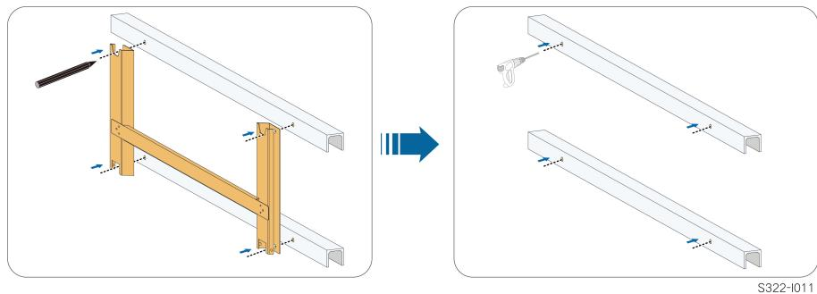
step 3 Secure the mounting-bracket with bolts.
