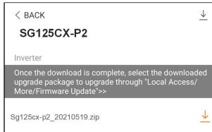
step 5 Return to the **Firmware Download** screen, tap
